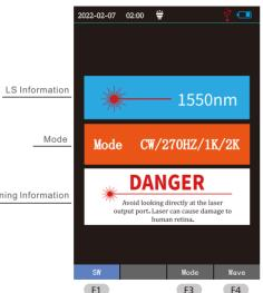
1310nm/1550nm light source and power meter display at the same time, convenient measurement
